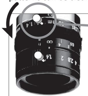
Gently unscrew the top lens lock screw on the camera in counterclockwise.
