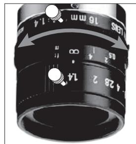
To adjust the focus, manually rotate the lens left or right until the geometric patterns can be seen clearly on the screen. After adjusting, gently lock the top lens by turning the lens lock screw in clockwise.
